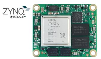
The EMC<sup>2</sup>-SoM also provides expansion for a VITA57.1 FMC<sup>TM</sup> LPC I/O board.
