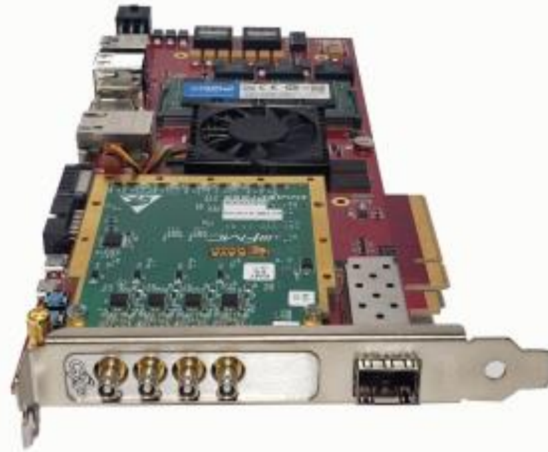
A FMC installed on a Sundance SE120 PCIe Carrier Board
