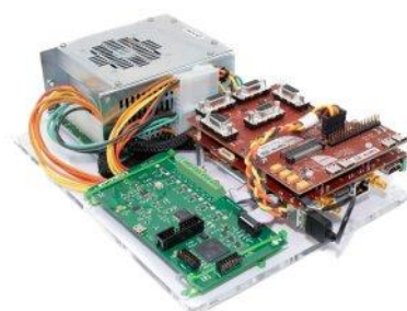
Photocaption 3: The TULIPP Starter Kit with Lynsyn PDM on a PC/104 carrier board.
