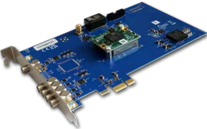
TimeTagger PCIe-Versions connect via PCIe x1 @ 400 MB/s
