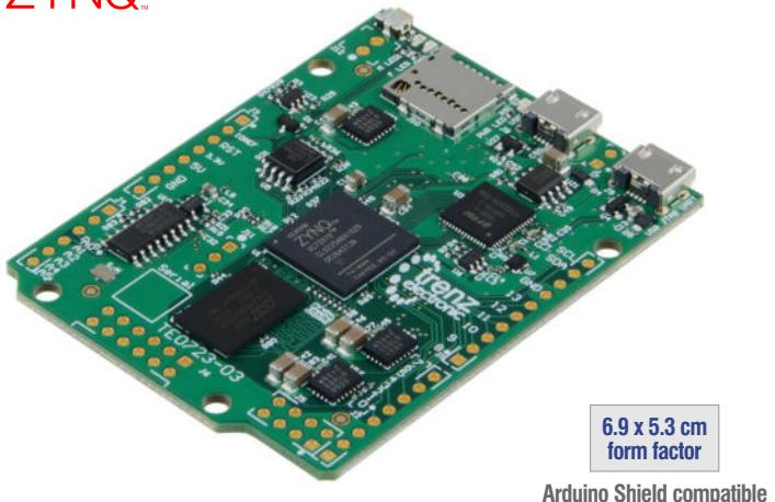
Arduino Shield compatible
