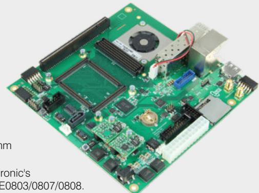
Designed for Trenz Electronic's TE080x MPSoC series TE0803/0807/0808.
