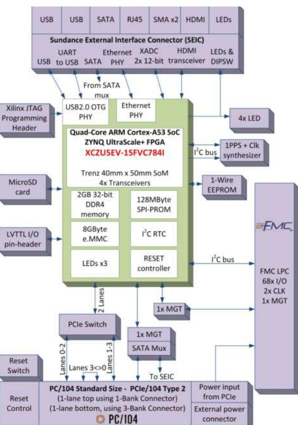
The EMC<sup>2</sup>-DP is a PCIe/104 OneBank™ Carrier for a Trenz compatible SoC Module and has expansion for a VITA57.1 FMC™ LPC I/O board. The SEIC board contains LEDs, RS232, USB2.0, HDMI, 1Gb Ethernet and SATA. It can be customised for individual applications and bespoke connectors. This provides a total solution for any embedded application.
