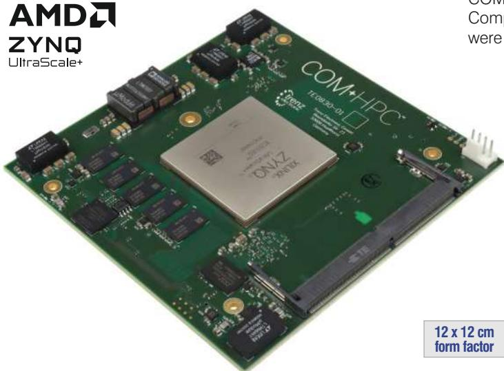
COM-HPC™ is the new released PICMG standard for high-performance Computer-on-Modules (COMs). The pinout and majority of the functionality were recently officially approved.
