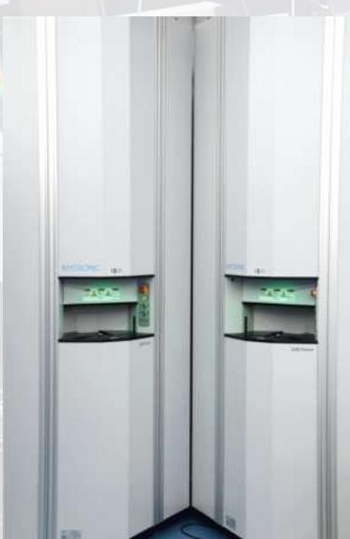
The modern, production-oriented storage system is an automated, highly flexible and expandable buffer storage unit for electronic components. It is ready for fast and smooth changeovers in our SMT line.
