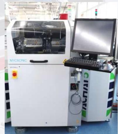
In the complex process of solder paste inspection (SPI), Trenz Electronic has the possibility to measure the paste volume with the highest precision in 3D. Furthermore, possible defects and bridges are detected.
