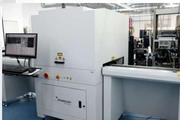
The Automatic Optical Inspection (AOI) is used to detect and report tolerance deviations in production using an image processing techniques.
