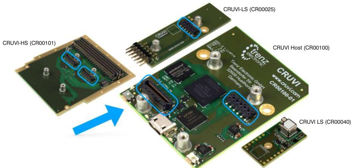
The picture shows FMC to CRUVI-HS, PMoD to CRUVI-LS, CRUVI Host with LS and HS slot and CRUVI LS modules.
