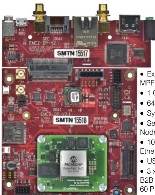
This system utilises a Microchip PolarFire® SoC MPFS250T, which is a low cost, small-sized FPGA module.
