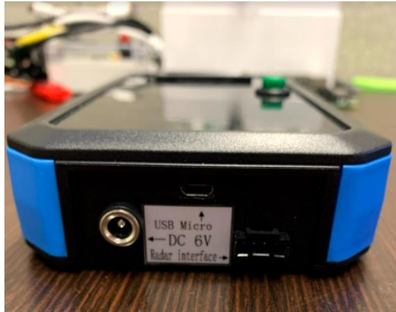
**Figure 12: US-D1 Firmware Update Board Connection**
