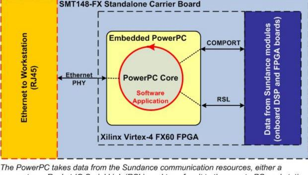
comport or a Rocket-IO Serial Link (RSL), and transfers it to the remote PC workstation using TCP/IP.
