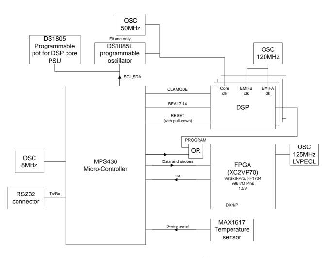
Starting at the top, the MPS430 is connected via an  $I^2C$  serial bus to a DS1805 programmable potentiometer. This pot is inserted into the DC-DC converter feedback, and thus can be used to adjust the DC-DC's output. The output is pre-set to 1.25V on power-up. The minimum value is 0.9V, and the maximum is above the Texas Instruments recommended voltage. Exceeding the absolute maximum voltage will cause damage to the DSPs.
