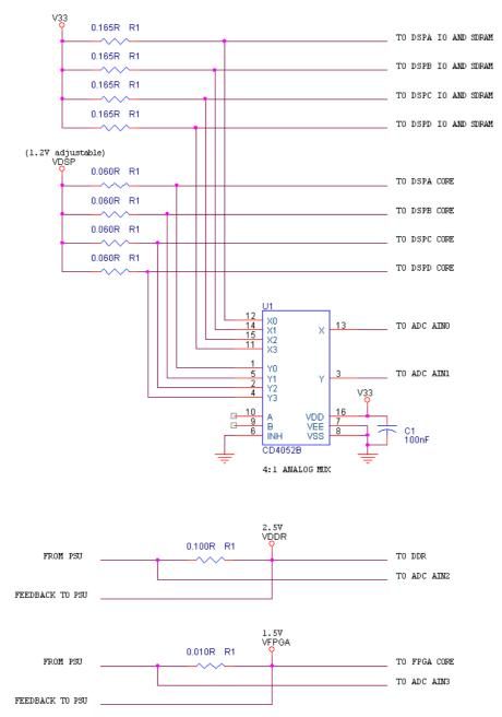
Series resistors are fitted inline with the output of the power supplies (DSP core and SDRAM) to be measured. The value of these is chosen so that the voltage drop will not exceed 5% under maximum load.
